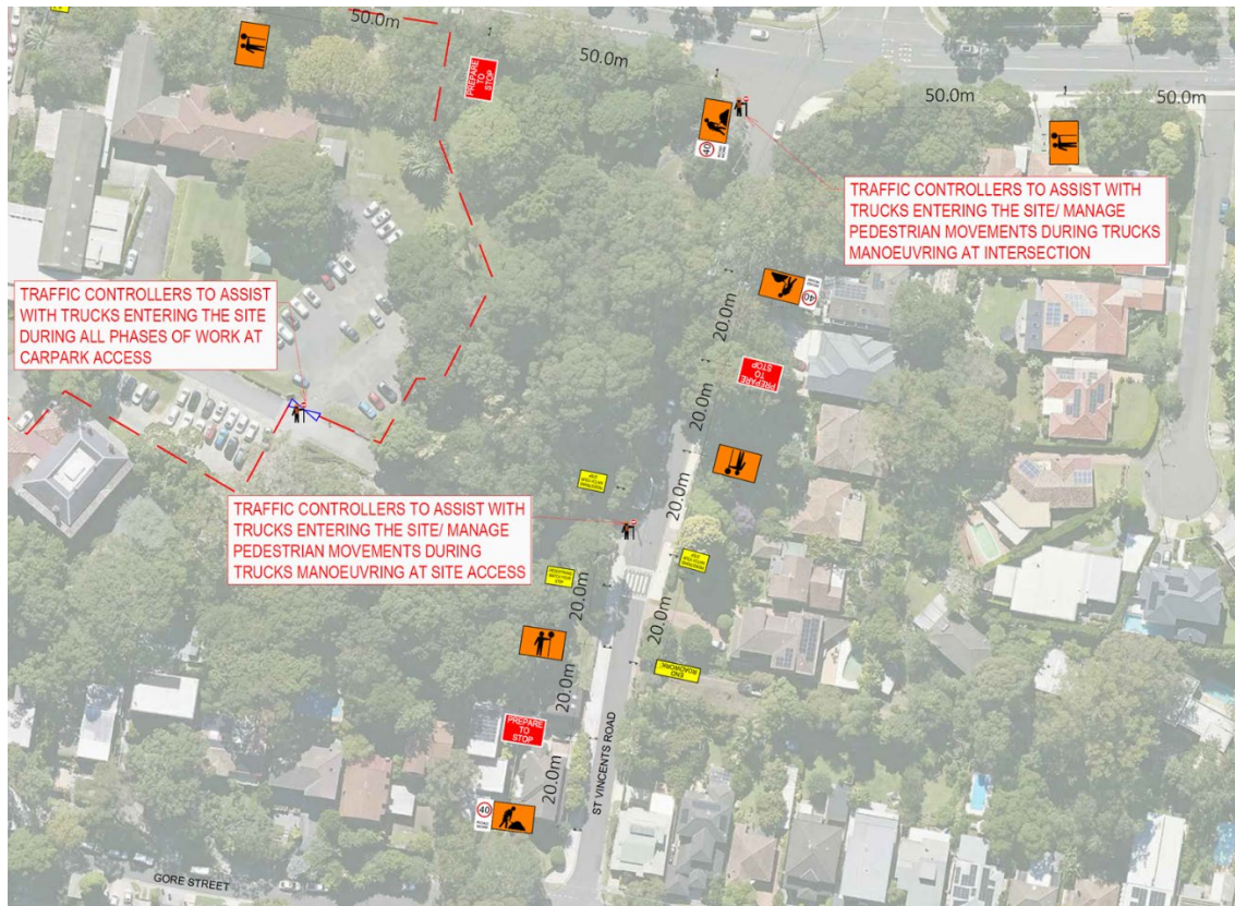
Figure 12 – Stage 2 Traffic Guidance Scheme St Vincents Road
